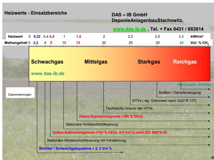
Figure 9 – Operation range of gas utilisation facilities
