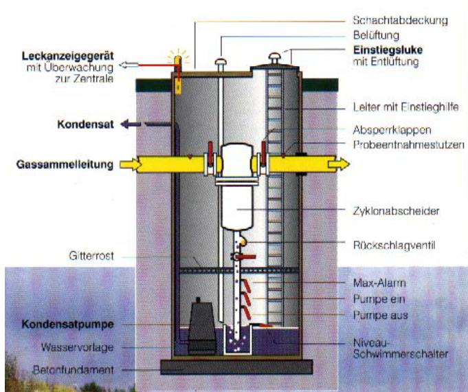
Figure 4– Condensate shaft
