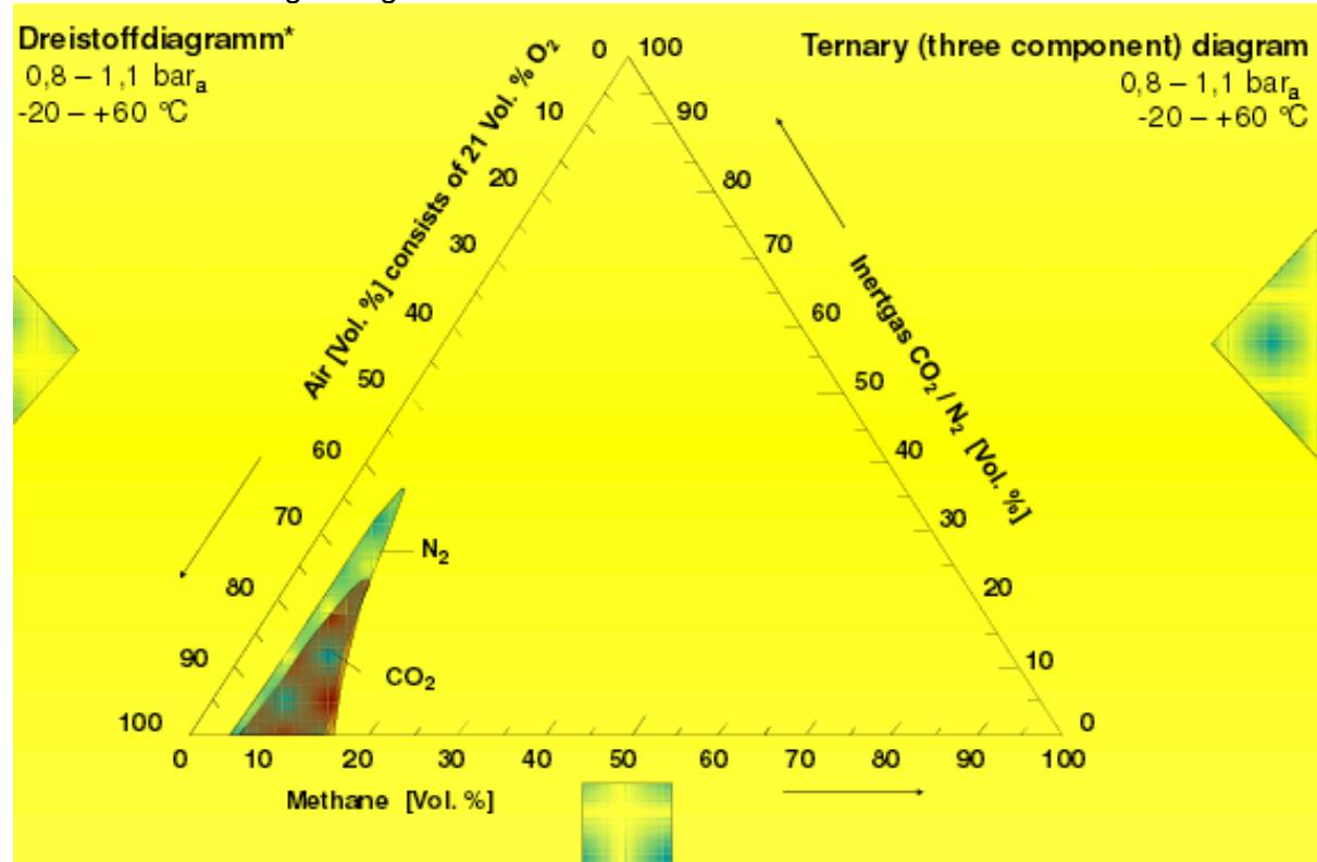
Figure 6 – Triangular explosion protection diagram,
