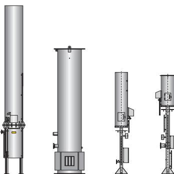
Figure 7 – Flare designs (from left: high temperate flare 1,200°C, 0.3s retention time to right: open "candle" flare without any emission standard)
