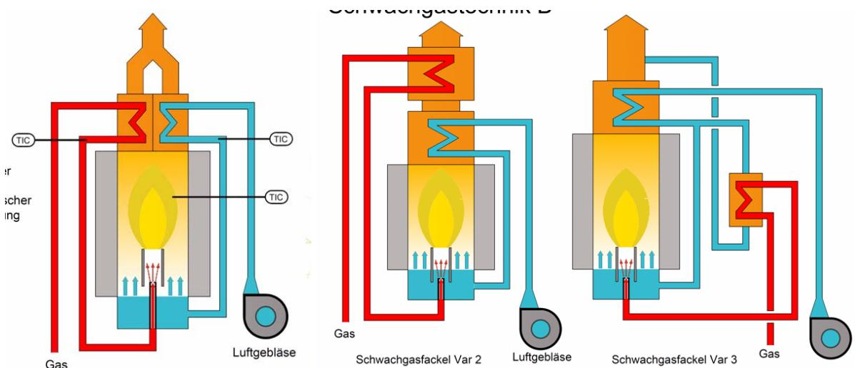
Figure 11 – Different heat exchanger systems for low calorific flares
