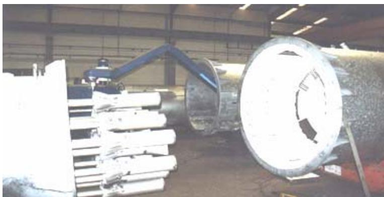
Figure 8 – Ceramic lining inside the flare stack (insulation liner)
